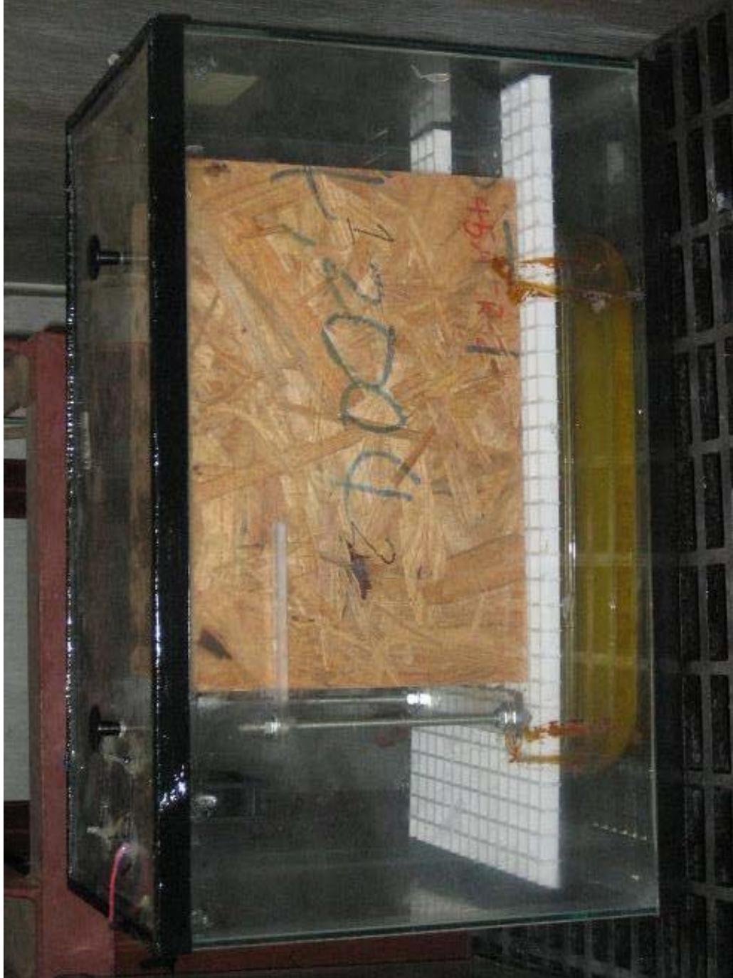
Figure 3.5. Relative humidity conditioning tank using saturate salt solution.
